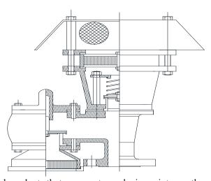
When storing flammable products or processing chemical products that can create explosive mixtures, the opening of the storage tank or vessel must be additionally protected with flame arresters. The task was to develop a device that combined the properties of a flame arrester and a valve into one design. PRECON® valves with integrated flame arrester units have the unique advantage that the flame arrester units are external and hence easily accessible.
